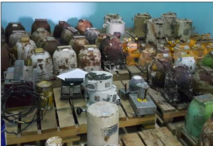
The DSRS are depicted here in their original containers that are bulky and deteriorated. These sources are usually stored in 200-litre drums.
