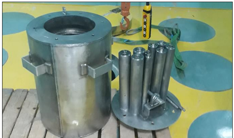
Once removed from the original devices, the DSRS are placed into specialised capsules and consolidated into specialised containers that increase safety, security and optimise storage space.
