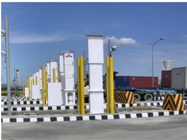
More than 10,000 radiation portal monitors (RPMs) and thousands more handheld detection devices are used around the world to detect illicit transport of nuclear and other radioactive material. (Source: Laem Chabang Port Customs Office)
