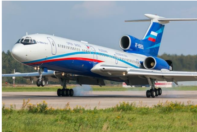
The Tupolev Tu-154M-LK-1 aircraft, converted for use as an Open Skies monitoring aircraft. Image Courtesy of: Dmitry Terekhov via Wikimedia Commons .
