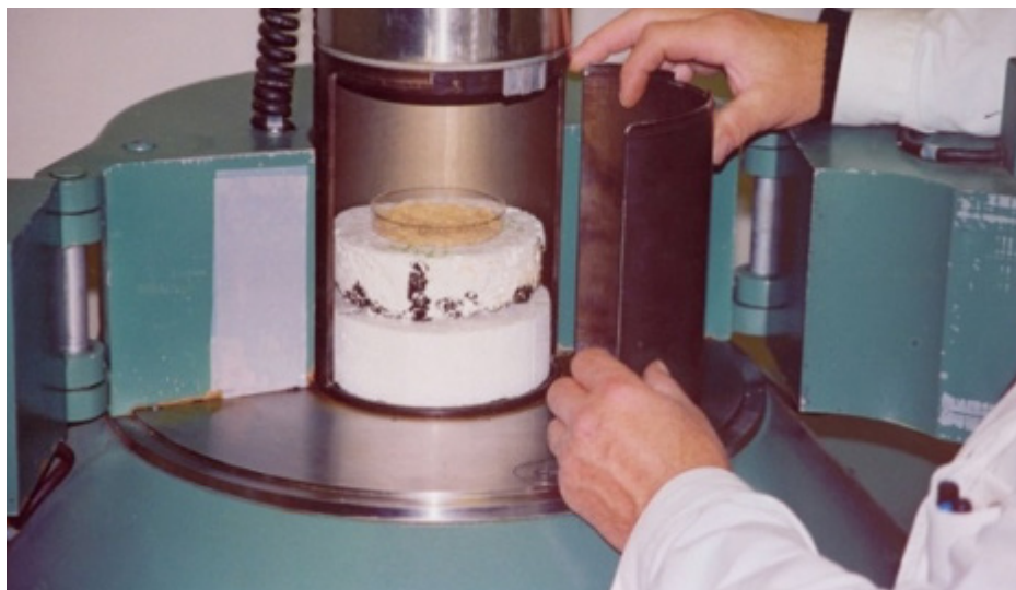
Gamma Cell (Cobalt-60) irradiating seeds at the FAO/IAEA Plant Breeding and Genetic Laboratory IAEA
