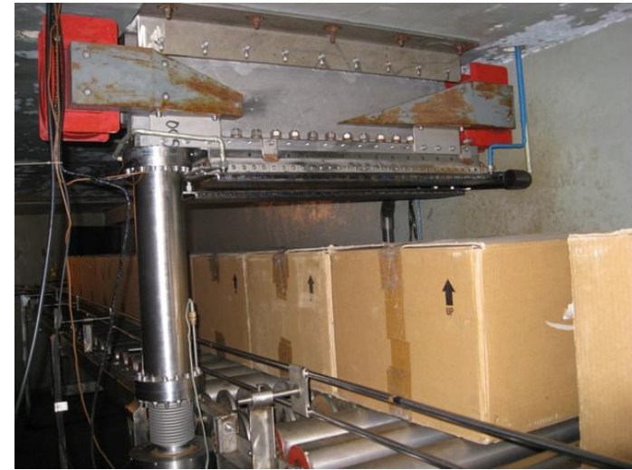
Model of EB irradiation using UERL-10-15S
