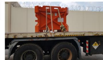
The DSRS packed in the licensed container ready for international transport. (Photo: IAEA Contractor)
