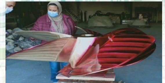
RT & PT on Marine propeller (service provided to JANNOT Group)
