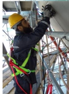
UT on chemical unit (service provided to Samir Oil Company)
