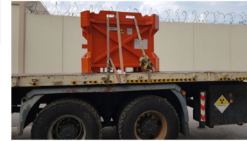
The DRSR packed in the licensed container ready for international transport. (Photo: IAEA Contractor)
