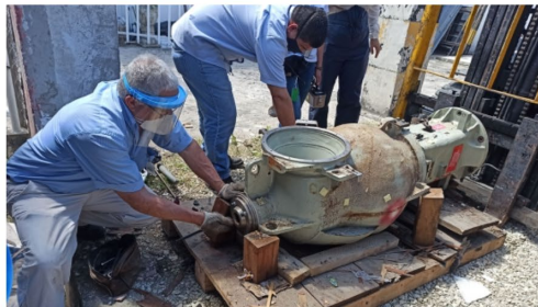
Experts dismantling a teletherapy head used for cancer care in Colombia in preparation for its safe and secure storage. (Photo: IAEA contractor)
