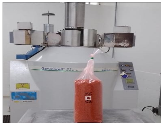
Fruit fly pupae sterilized using a gamma irradiator at the Guatemala insect mass rearing and sterilization facility, which produces 1.2 billion sterile medflies a week. Photo credit: Dr Pedro Redon/MOSCAMED - Guatemala.
